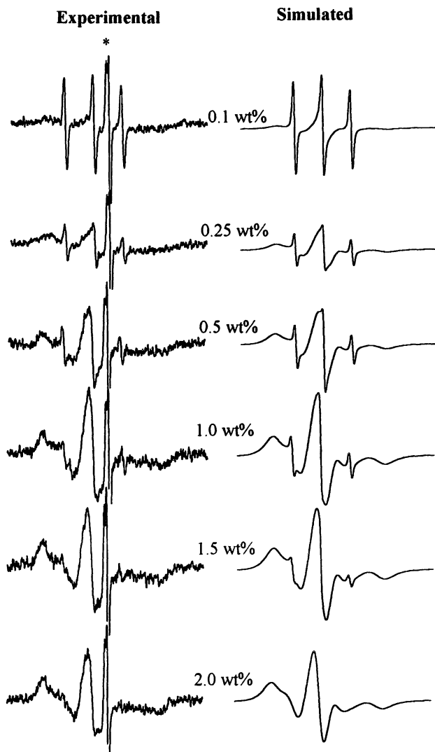
Figure 5. Effect of Silica amount on EPR spectra of HTAB*. All samples are at pH=7 and 10^{-4} M HTAB*. Spectra simulated with HTAB* in solution (rapidly rotating) and HTAB* on the silica surface (slowly rotating).
